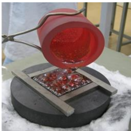
Sintering of frit/nanographite mixture
