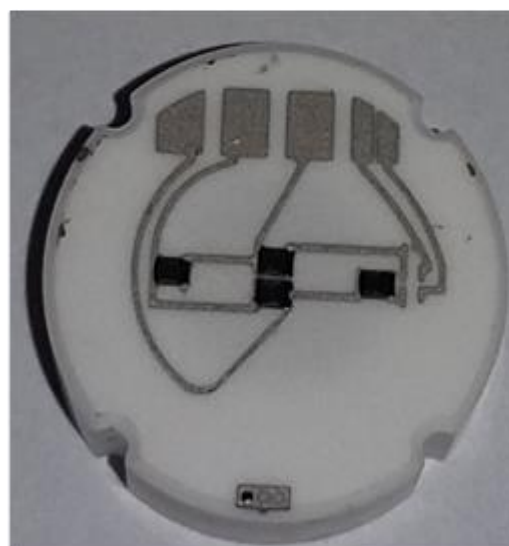
Pressure sensor in Wheatstone bridge configuration
